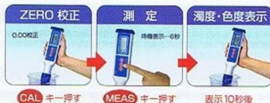
**モード切換えで最小0.1→0.01度の切換え表示**
